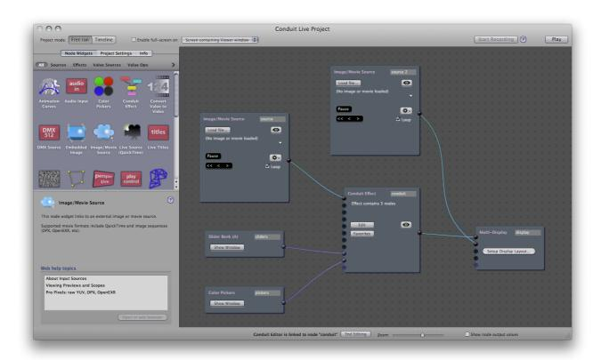
On the right-hand side of the Project window, we see boxes interconnected by cyan and purple lines. These represent the different "devices" within the control room. The connections between the devices are like electric wires that transmit signals from one device to another. As in the real world, some of these wires carry video and others carry control signals. The color of the wire indicates the type of content.
