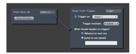
In the above screenshot, the Trigger node has been set to trigger cues based on the connected *Slider 1*. When the user moves Slider 1 above the "trigger treshold" of 0.01, the next cue in the Stage Tools cue list will be triggered.
